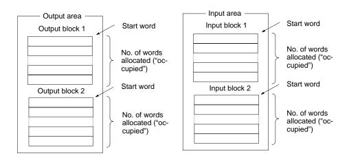
**Note** Using a Configurator, set the areas for each block, the start word, and the allocated words for each block.
